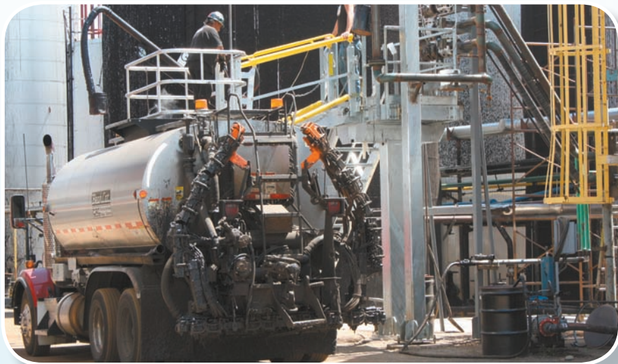
A BearCat distributor takes on a load of polymer-modified asphalt emulsion at the VSS Emultech plant.
