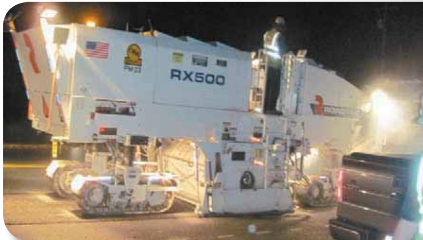
A ROADTEC RX500 is used by C.W. Matthews Contracting to mill pavement during night project in Stockbridge, Ga.
