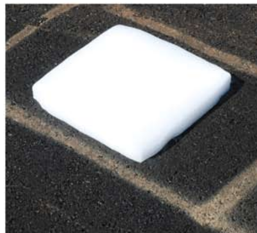
On a sunny spring afternoon, dry ice chills the hot mat in advance of coring. The core samples of the Oklahoma I-40 HiMA mat will be analyzed in labs across the United States.
