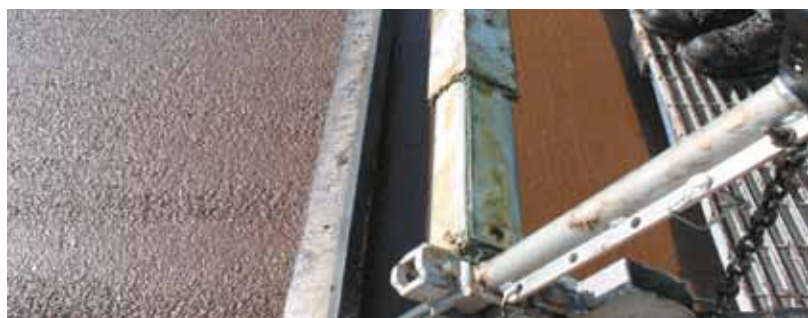
A plate mounted behind the screed produces a textured micro surface (at left).
