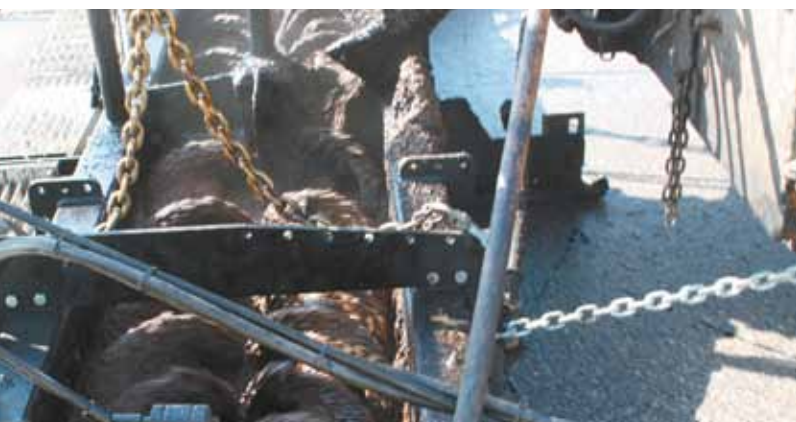
Augers blend ingredients before material exits the micro surfacing machine.
