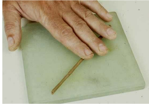
Figure 31. Photo. Plasticity test.
