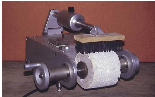
Figure 55. Photo. Abrasion resistance test.
