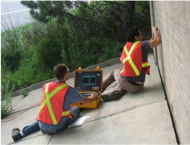
Figure 7.12. Non-destructive testing of ASR-affected concrete structures. A. Impact-echo. B. Non-linear acoustic technique.
