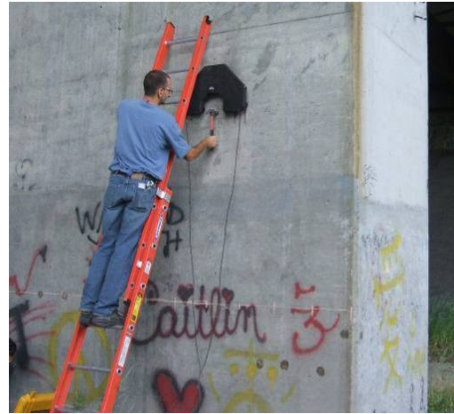
Figure 7.12. Non-destructive testing of ASR-affected concrete structures. A. Impact-echo. B. Non-linear acoustic technique.
