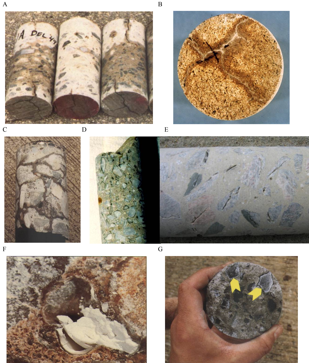
Figure 7.5. Macroscopic observations on cores (as received condition). A. Cores extracted from a concrete pavement affected by ASR and showing macrocracks penetrating from the upper and lower parts of the pavement. B. Gel staining surrounding cracks and gel exudations at the surface of a core extracted from a sidewalk section affected by ASR. C. Fine cracking pattern showing up after re-wetting of the core. D. Dark rim surrounding reactive aggregate particles. E. Macrocracks in reactive coarse aggregate particles. F. Deposits of alkali-silica gel in a void on core surface. G. Deposits of alkali-silica reaction products on the broken surface of a core extracted from a highway bridge structures affected by ASR.
