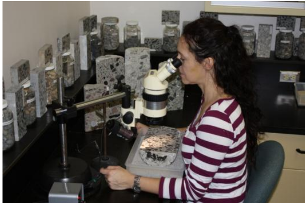
Figure 7.13. Examination of the polished concrete section under the stereomicroscope for the determination of the Damage Rating Index . Petrographic features of deterioration (Table 7.8; Figure 7.7) are counted in a one cm x one cm grid system drawn at the surface of the polished concrete section.
