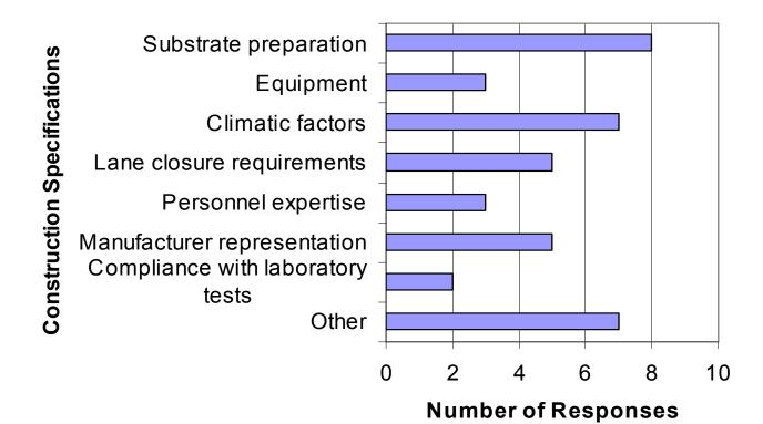
• Substrate preparation applied to repairs, climatic factors were usually minimum temperatures, and manufacturer representation generally involved 1 to 3 days of inspection
