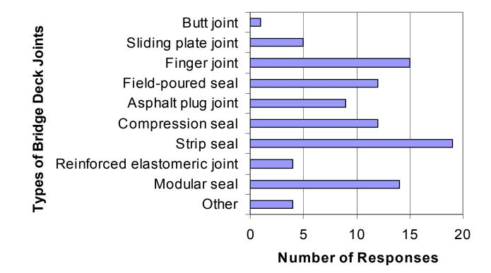
• Strip seals were most accepted type of joint, followed by finger joints
