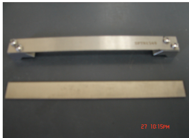
Figure 11 Calibration Beam: In the Front, Compliance Beam for SuperPave™ BBR Test and in the Back, Modified Compliance Beam for Crack Sealant BBR Test
