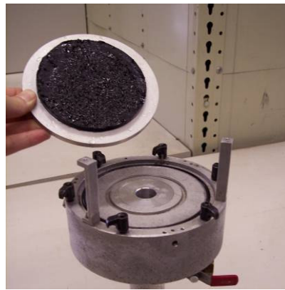
Figure 17. Place the first specimen on the base setup
