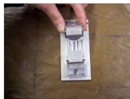
Figure 4. Place two end pieces on the mold
