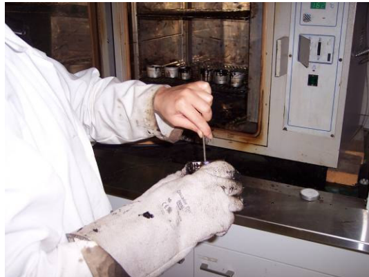
Figure 2. Remove the can, mix the sealant thoroughly and place it back in the oven for another 15 minutes
