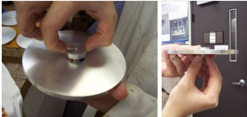
Figure 5. Place the plug on the annular plate, and pull it from underneath the plate until it fits in the orifice and the film edges sits on the plate
