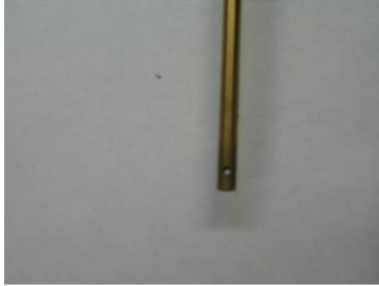
Figure 2. Lower opening of 2.5mm to screw the spindle to the rigid rod
