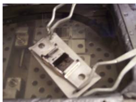
Figure 11. Grab the base plate with two tongs and place it in cooling bath
