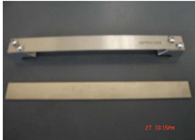
Figure 11. Calibration Beam: In the Front, Compliance Beam for SuperPave™ BBR Test and in the Back, Modified Compliance Beam for Crack Sealant BBR Test
