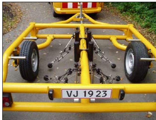
The open CPX noise trailer "decibelA" from the Danish Road Institute.
