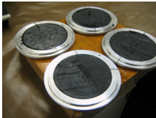
Figure 9. Let the sealant set for one hour at room temperature
