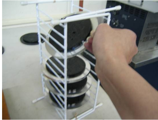
Figure 13. Place the plated on the rack; allow enough clearance between each two specimens
