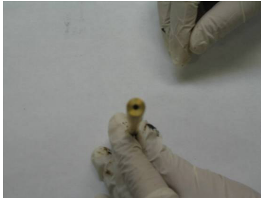
Figure 3. Upper opening of 2.5mm to screw the rod to the viscometer head
