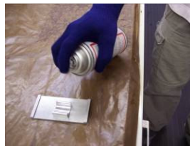
Figure 3. Spray release agent on the mold
