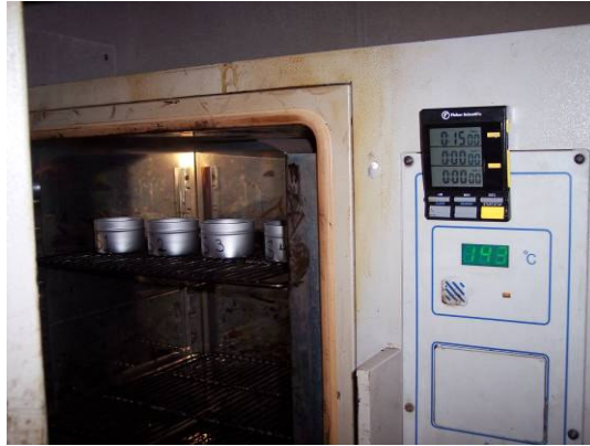
Figure 1. Heat 35 gram of homogenized sealant at recommended pouring temperature for 30 minutes
