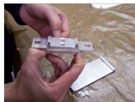
Figure 5. Hold the assembly in place using a rubber band
