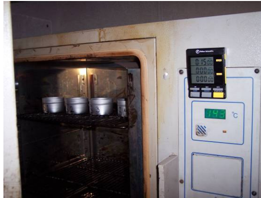
Figure 1. Heat four cans of 80g homogenized sealant for 15 minutes at the recommended pouring temperature
