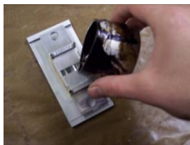
Figure 8. Remove the sealant from the oven and mix thoroughly and pour it in the mold from one corner
