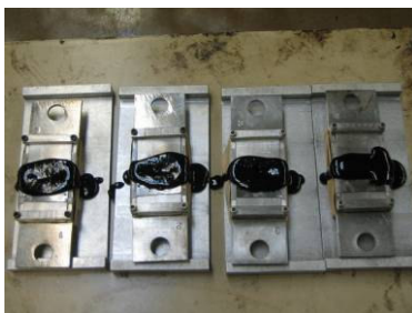
Figure 9. Let sealant set for one hour at room temperature
