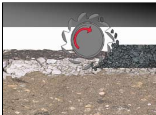
Schematic of a milling machine processing an asphalt pavement.
