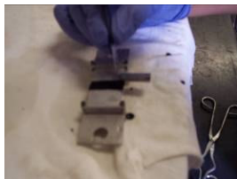
Figure 18. Flip back the specimen and push the notch horizontally until it comes off
