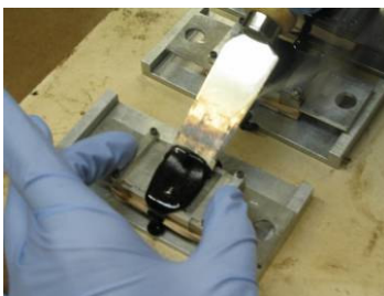
Figure 10. Trim the extra sealant away using a heated spatula
