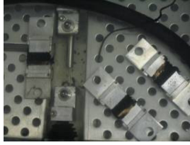
Figure 20. Leave the specimens for 45 minutes in the bath
