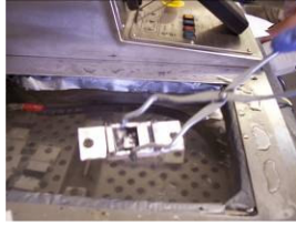
Figure 14. Remove one specimen at a time holding its center using a tang
