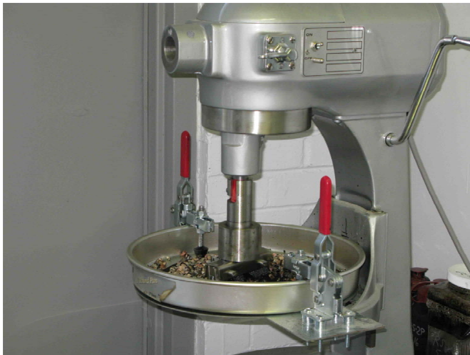
Figure 4. Modified Sweep Test Mixer
