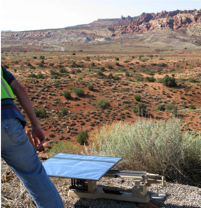
Figure 5. Moisture Test Pads Prior to Spraying/Chipping
