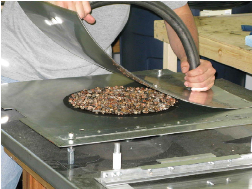
Figure 3. Compactor Setting Aggregates on Test Pad
