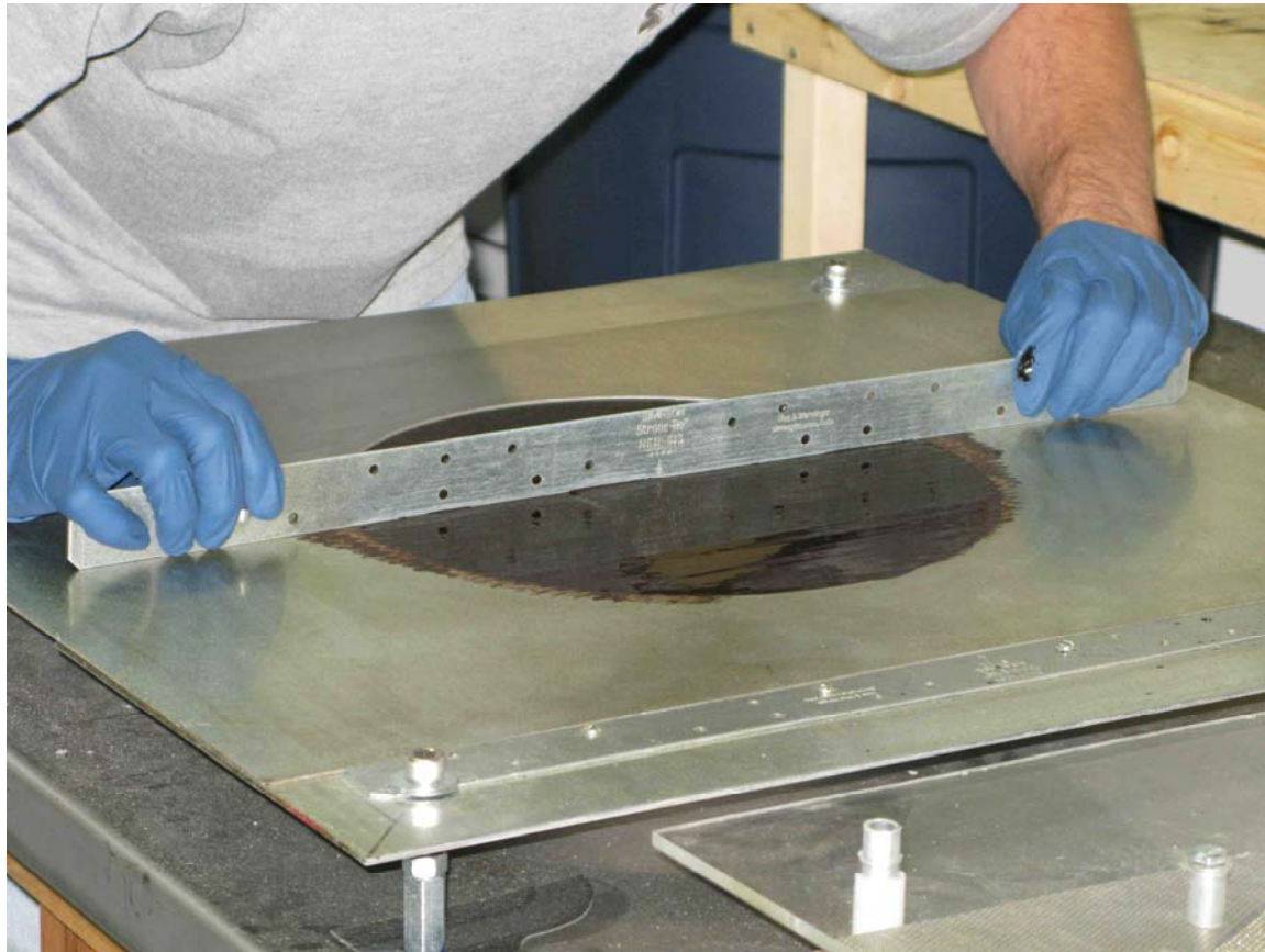
Figure 7—Emulsion Strike-Off In Template
