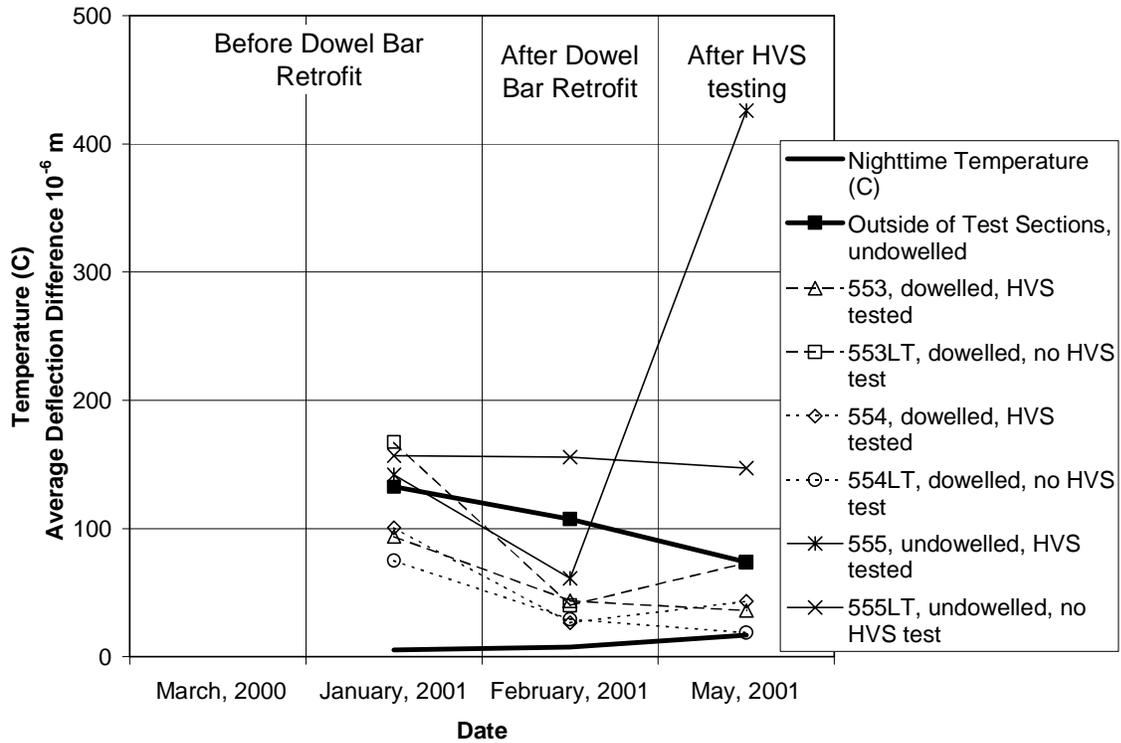
**FIGURE 9 Comparison of deflection difference between slabs for nighttime measured with the Falling Weight Deflectometer on all HVS test sections and “outside” control section before and after HVS trafficking.**
