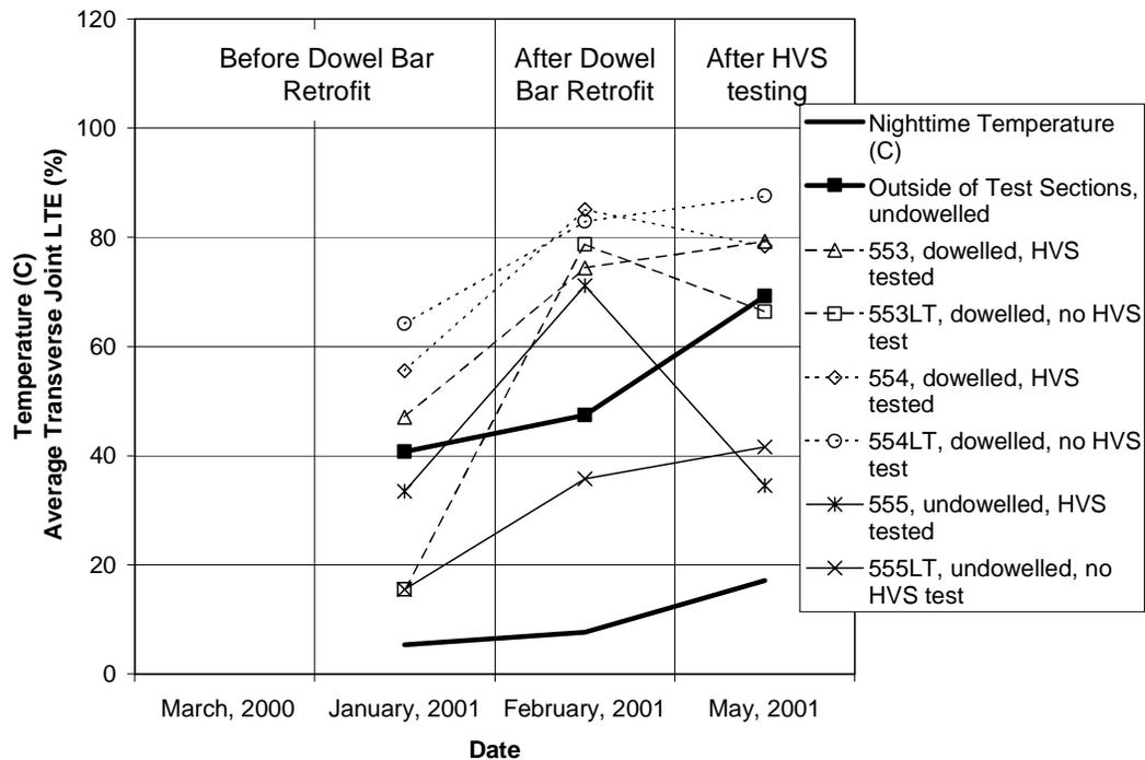
**FIGURE 8 Comparison of load transfer efficiency for daytime (8a – top) and nighttime (8b – bottom) measured with the Falling Weight Deflectometer on all HVS test sections and “outside” control section before and after HVS trafficking.**
