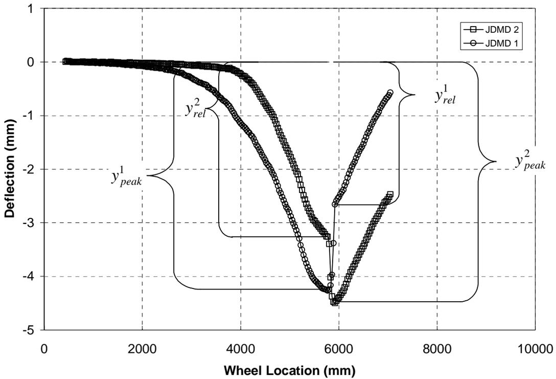
FIGURE 2 Example of LTE calculation from JDMD measurements.
