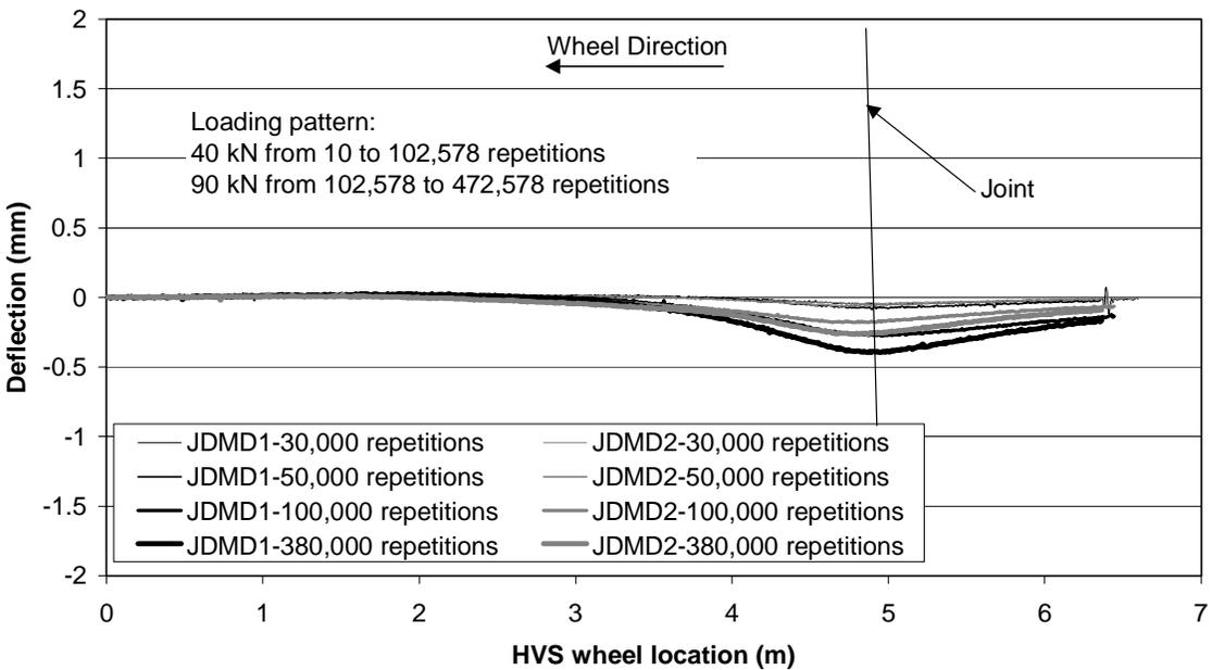
**FIGURE 4 Influence lines for JDMDs 1 and 2 versus load repetitions under HVS loading on Sections 555FD (4a - top) and 554FD (4b - bottom).**
