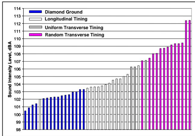
**Figure 3. Overall A-weighted Sound Intensity Levels of Tire/Pavement Noise for Concrete Surfaces – Calif./Ariz. database with indicated groupings.**
