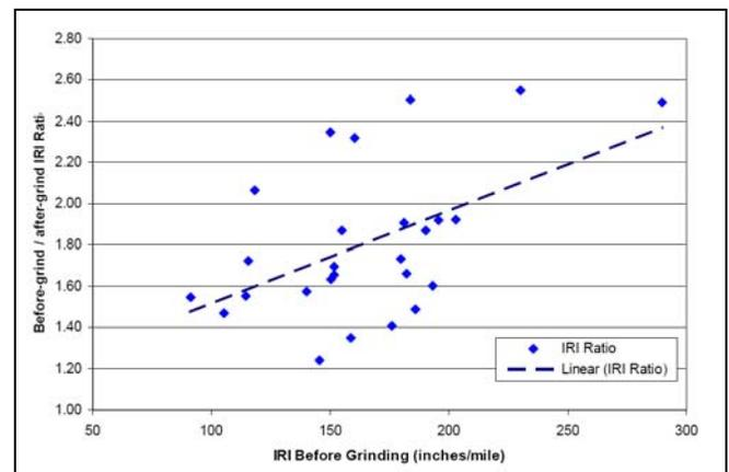
Figure 1. Improvement in Ride Quality (shown as the Ratio of Before-Grind IRI and After-Grind IRI) versus IRI Before Grinding.
