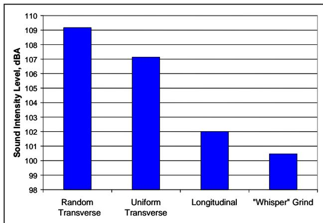
**Figure 4. Sound Intensity Levels for Different Concrete Pavement Textures in Arizona.**
