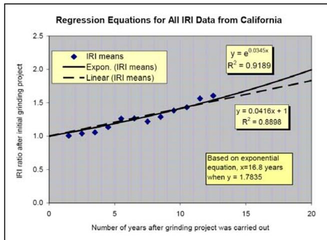
**Figure 2. Change in Smoothness from Initial Post-Grind IRI versus Time.**
