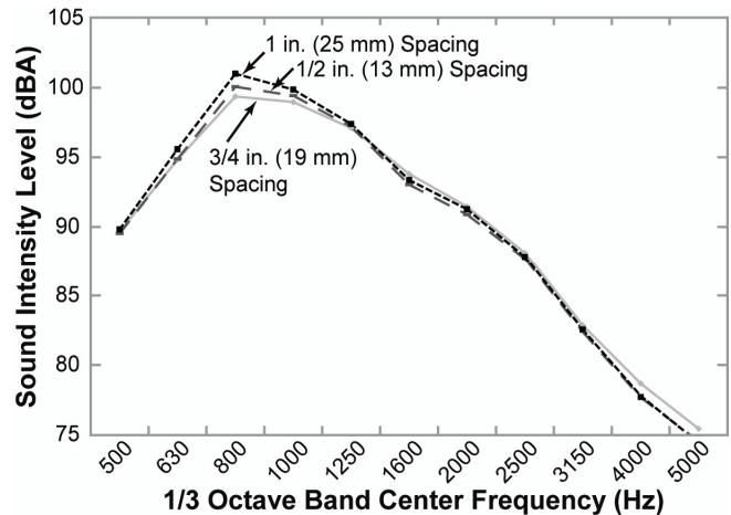
**Figure 4.** Evaluation of groove spacing effect on OBSI spectral plots for a 1/8 in. (3.2 mm) standard groove at various spacings.
