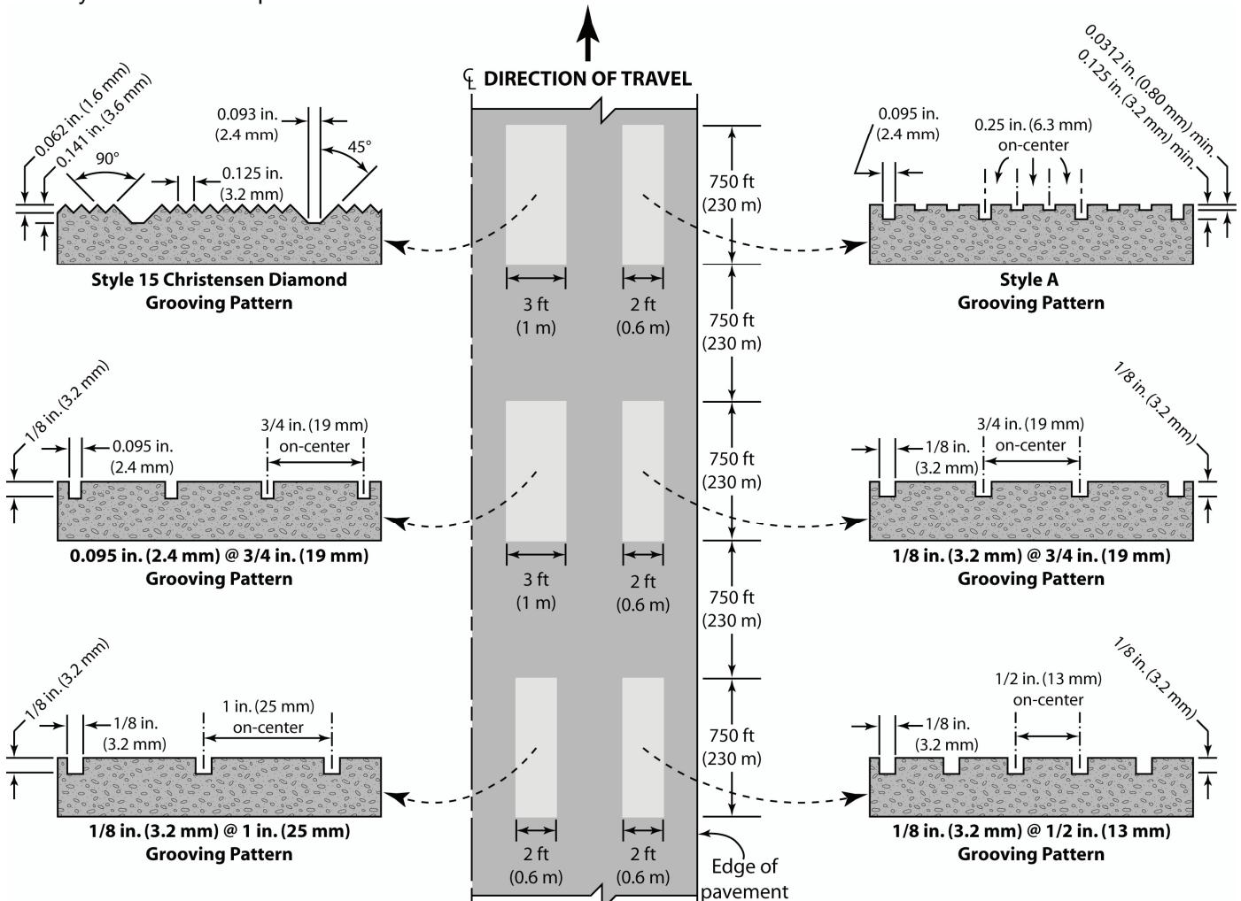
**Figure 1.** Layout and grooving patterns for the six diamond grooving test sections in the 1969 Caltrans diamond grooving experiment on County Road 32A.
