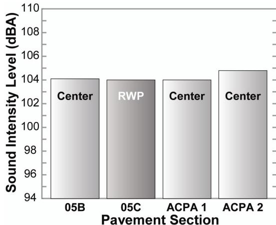
**Figure 2.** Comparison of OBSI test results for drag texture in the right wheelpath (RWP) and between wheel paths (Center). Detailed information on the test section locations is available in reference 2.
