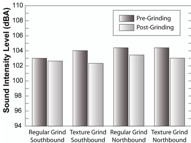
**Figure 6.** Comparison of overall OBSI levels for sections with original and two types of diamond ground textures<sup>6</sup>.
