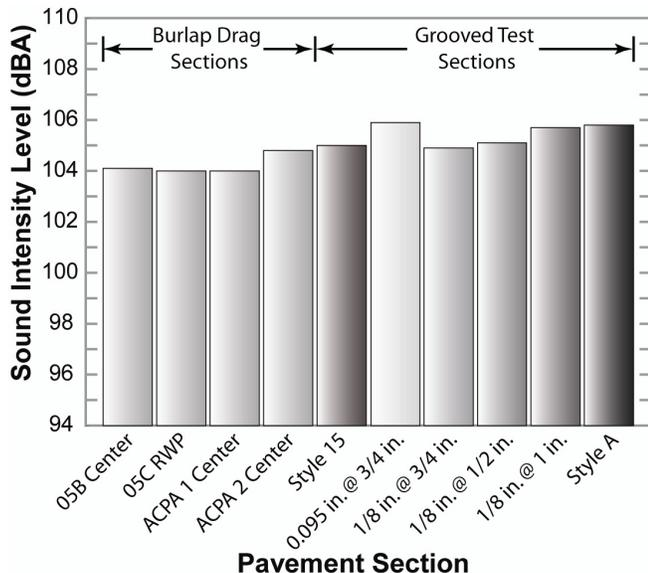
**Figure 3.** Comparison of OBSI test results for the burlap drag textures and all six grooved sections.
