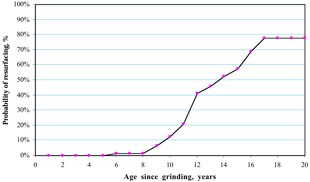
Figure 15. Survival curve showing probability of resurfacing (overlying, reconstruction, or regrinding) vs. age since first grind for diamond-ground pavements.
