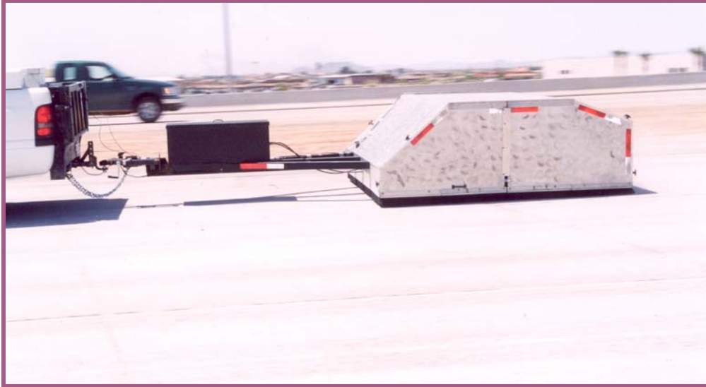
Photo depicts trailer equipped with instruments to measure tire/pavement noise using the close-proximity or CPX method. The CPX method, which measures noise at the tire/pavement interface, was used by the Arizona DOT, which measured diamond ground pavements and found tire/pavement noise was reduced significantly. (Photo: Bill Davenport, ACPA)
