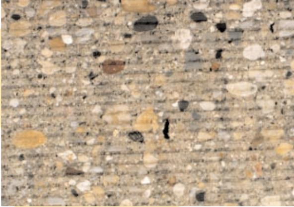
*Diamond ground surfaces are proving to be the quietest concrete pavements.*
