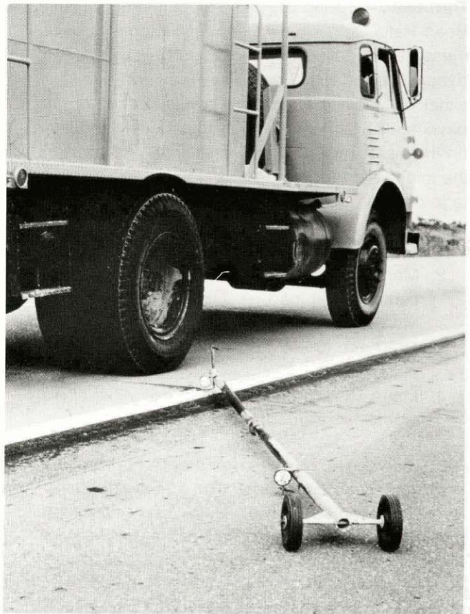
Figure 2 Static load deflection test using a Benkelman beam.
