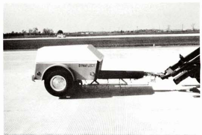
Dynamic Load Deflection Devices: (Top) Falling Weight Deflectometer (Bottom) Dynaflect.
