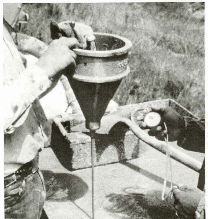
Figure 8 (Top) Cross section of a flow cone. (Bottom) Grout discharge and timing check.
