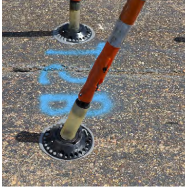
Figure A-4. Sample 2B Failure at 44 Impacts.
