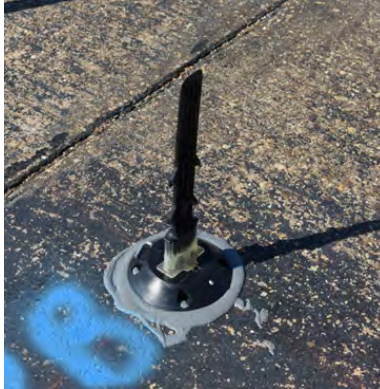
Figure A-14. Sample 7B Failure at 18 Impacts.
