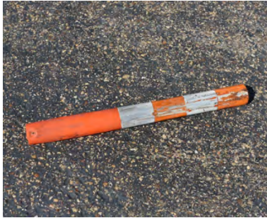
Figure A-2. Sample 1B Failure at 27 Impacts.
