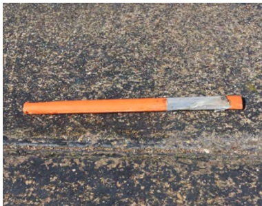
Figure A-16. Sample 8B Failure at 28 Impacts.
