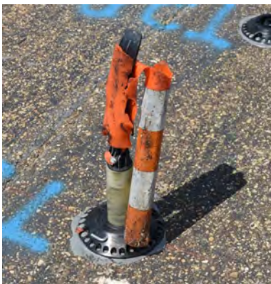
Figure A-5. Sample 3T Failure at 71 Impacts.
