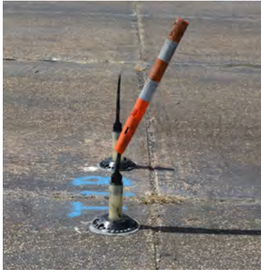
Figure A-1. Sample 1T Failure at 53 Impacts.
