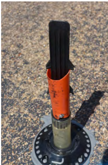
Figure A-8. Sample 4B Failure at 42 Impacts.
