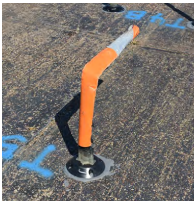
Figure A-9. Sample 5T Failure at 32 Impacts.
