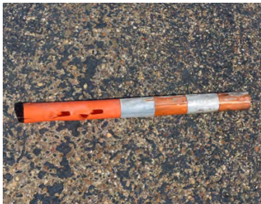
Figure A-6. Sample 3B Failure at 28 Impacts.
