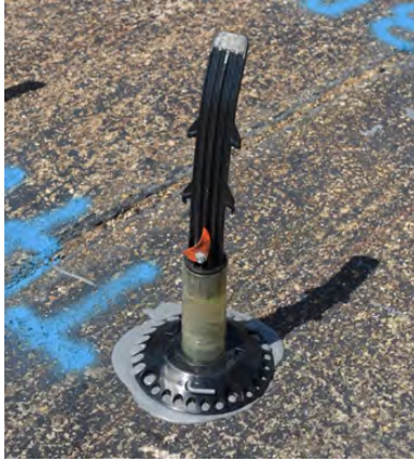
Figure A-7. Sample 4T Failure at 56 Impacts.
