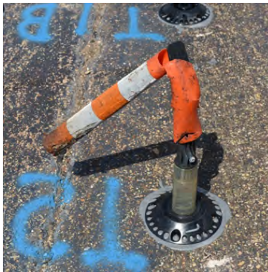
Figure A-3. Sample 2T Failure at 66 Impacts.
