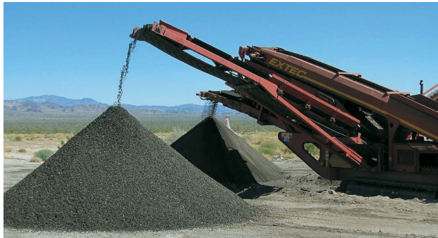
Crushing and screening of RAP into usable fractions creates an engineered product from one-time waste material, permitting blended stockpiles with consistent residual asphalt content which can be figured into mix designs
