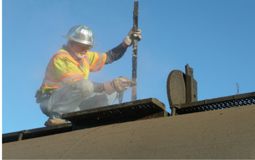
Figure 29: Recording Initial Tank Volume with Dipstick
