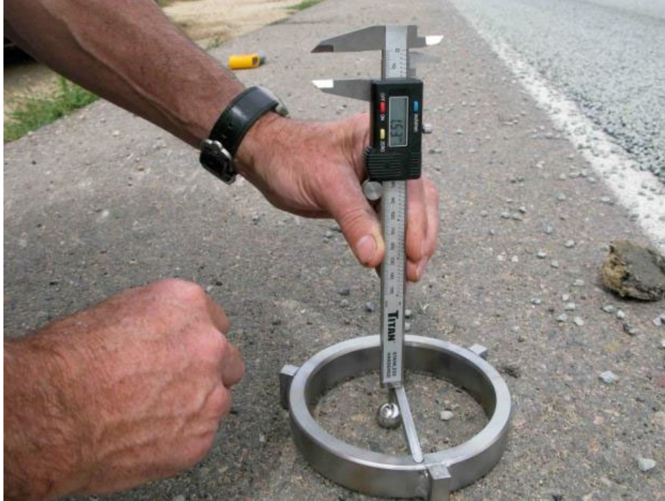
Figure 14: Ball Penetration Test
