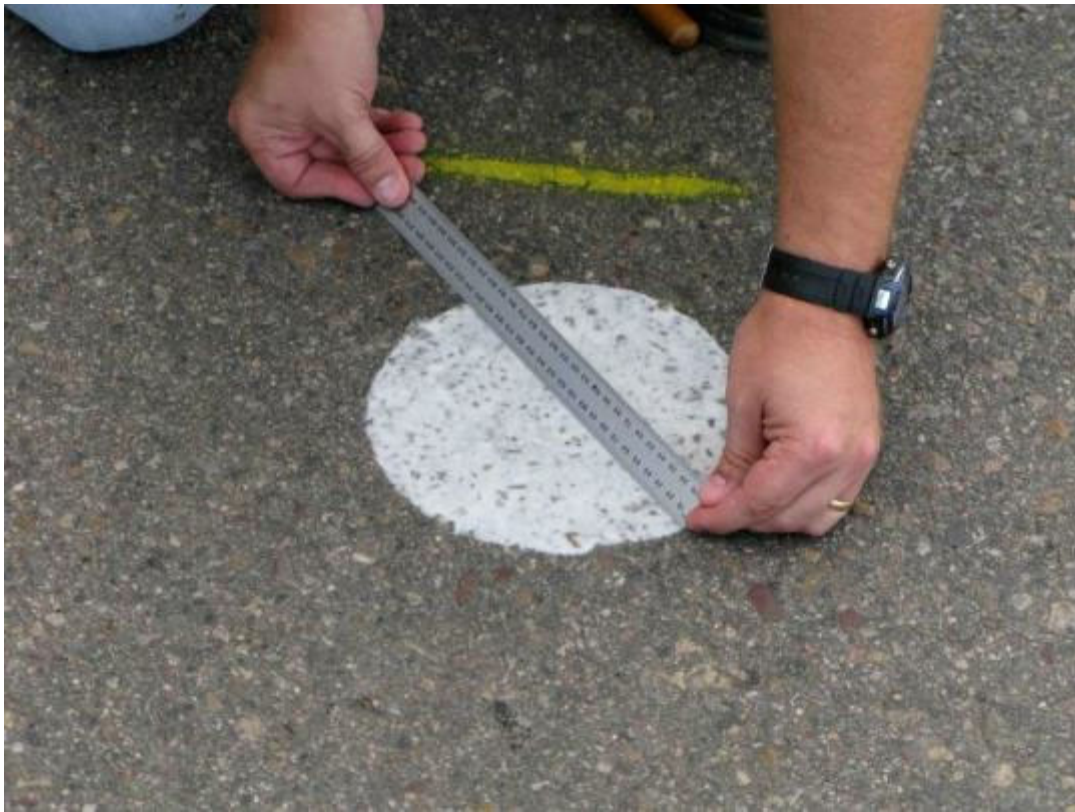
Figure 13: Sand Patch Test Method
