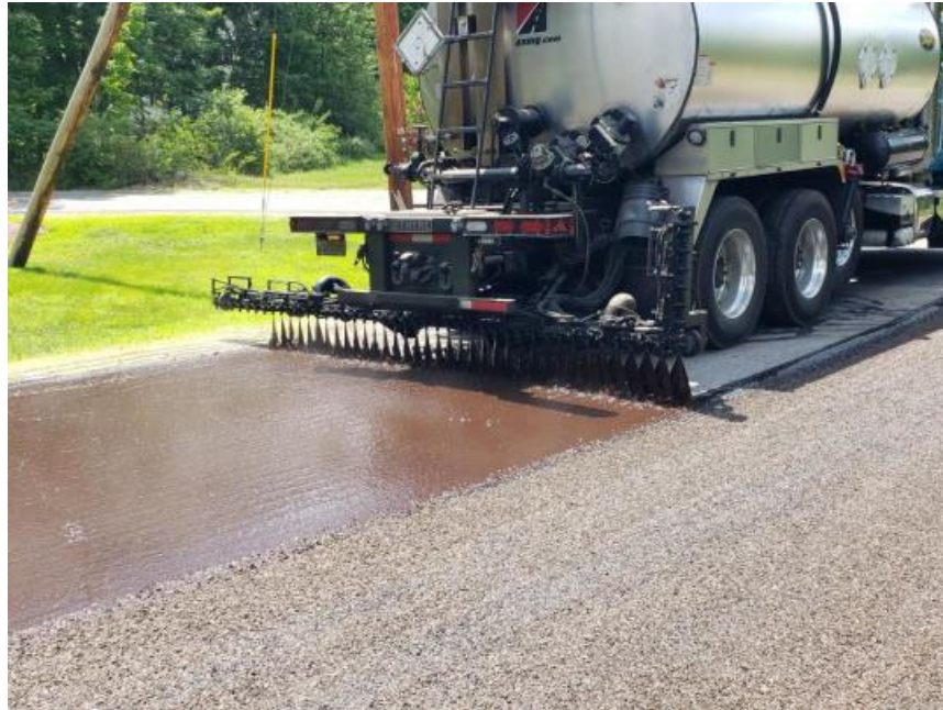
Figure 18: Typical Asphalt Distributor
