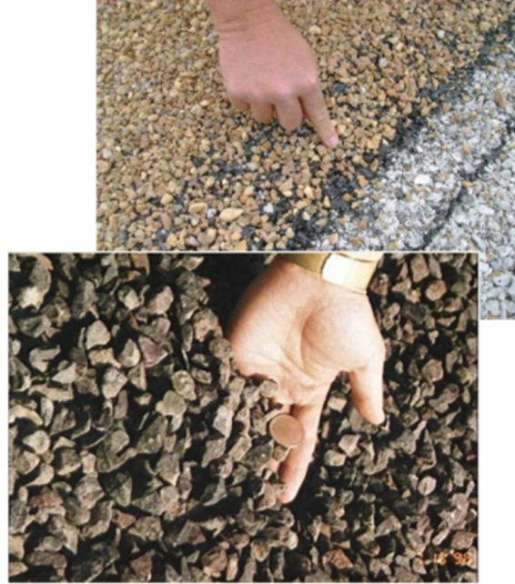
Figure 11: Round and Angular Aggregates
