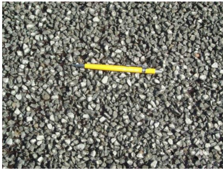
Figure 34: Appearance of Aggregate in Emulsified Asphalt Before Rolling
