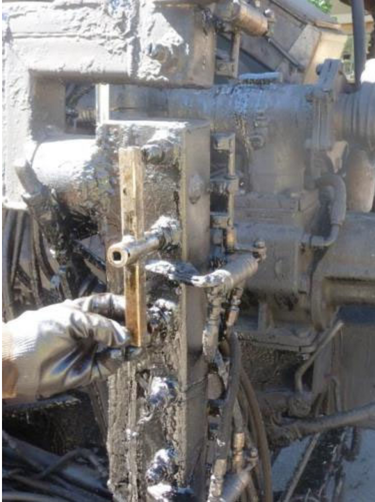
Figure 21: Adjusting Nozzle Angle with Nozzle Wrench
