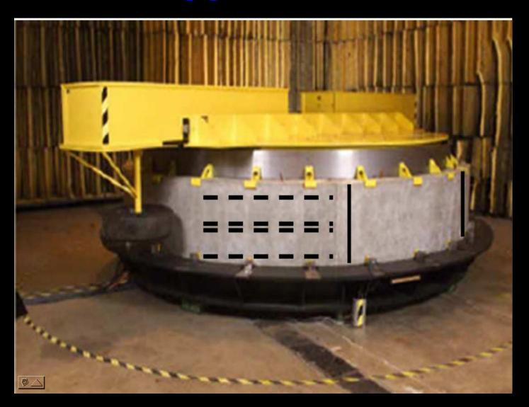
Why Use the Purdue Tire Pavement Test Apparatus (TPTA)
