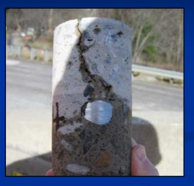
Full Depth Cracking is apparent Avg. Cracking – 0.006 – 0.010 in. Some as large as 0.014 in. Within 2- 3 SF areas
