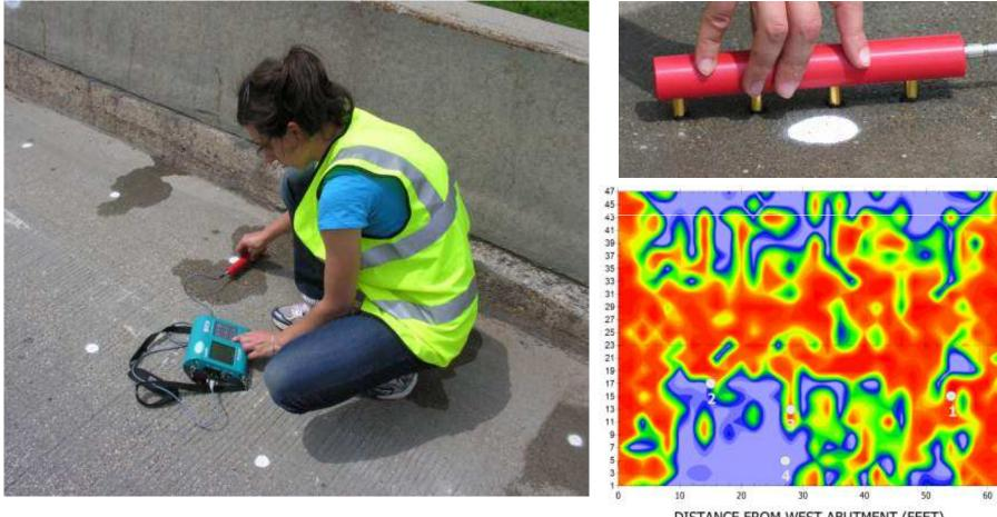
DISTANCE FROM WEST ABUTMENT (FEET) Electrical Resistivity, kohm/cm
