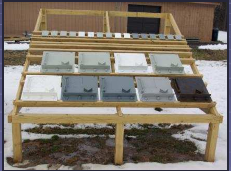
Natural Weathering without Salt Spray
